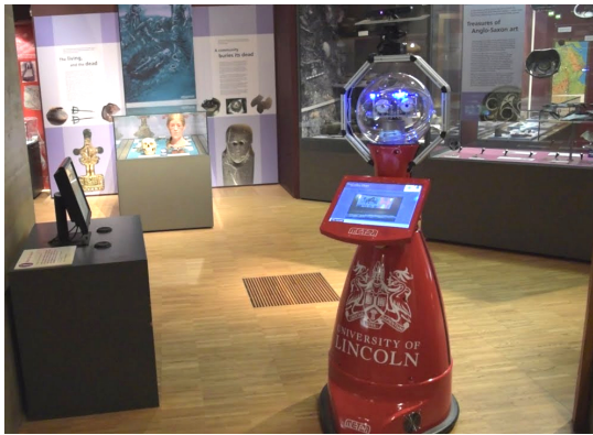
Fig. 1. Lindsey, the mobile robot deployed as a tour guide in the Lincoln Museum.
